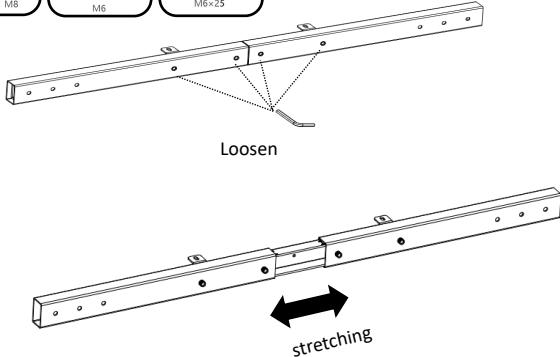
Loosen 4 screws with M8 hex key (A) and then pull the beam (4) apart
