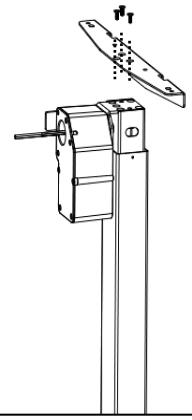
Put the two columns (2, 3) upside down on the ground with a distance between them; Connect the bracket (6) with the left and right columns (2, 3) with m6x20 screws (E) and lock it with M6 hexagon key (A).
