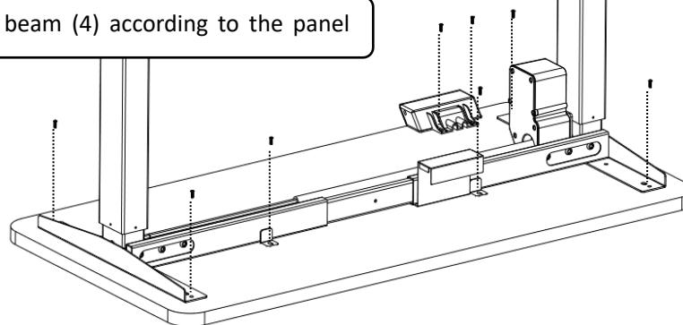
Tighten the panel and hand controller (10) with self tapping screw st4.8 (B)
