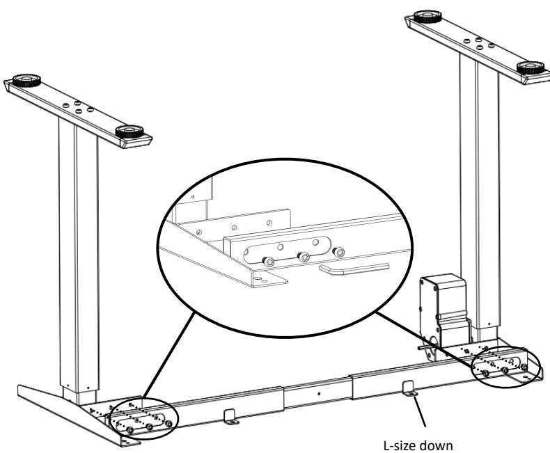
Place the cross beam (4) upside down, connect it with the column (2, 3) with m8x10 screw (C), and lock it with M8 hexagon key (A).
