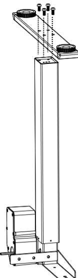
Place the two feet (1) on the left and right columns (2, 3), connect them with m8x30 screws (D) and lock them with M8 hexagon key (A).
